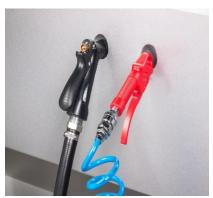
**Air Gun and Coolant Gun** are conveniently located below the control panel . They are provided for blowing away chips embedded inside work piece holes and pockets as well as washing away chips piling up along the sides of the table.
